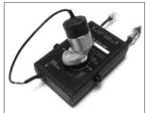
Figure 3. Hearing instrument positioning for TMFS testing with BTE (top) and ITE/ITC (bottom) instruments.
