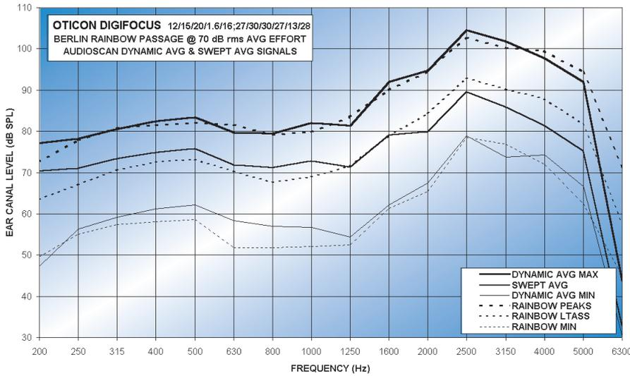
Meeting gain targets using steady pure tones or broad-band noise will frequently not result in the 1/3 octave band levels of amplified speech reaching expected levels. Audioscan has dealt with this problem with two unique time-varying signals – a swept burst-biased tone (SWEPT) and a roving bilevel tone (DYNAMIC).
